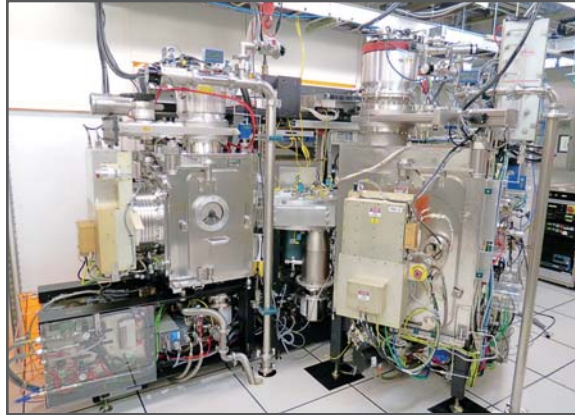
Veeco IBD/IBE (Ion Beam Deposition & Etch) w/CX6C2 Metal Film PVD Sputtering System w/Etch Mill Module
