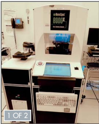
Nanometrics NanoSpec 8000X Model 7000-0493 Rev-P1 Film Thickness Analyzer/Measurement Systems
