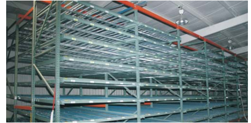
GRAVITY FLOW RACKING
